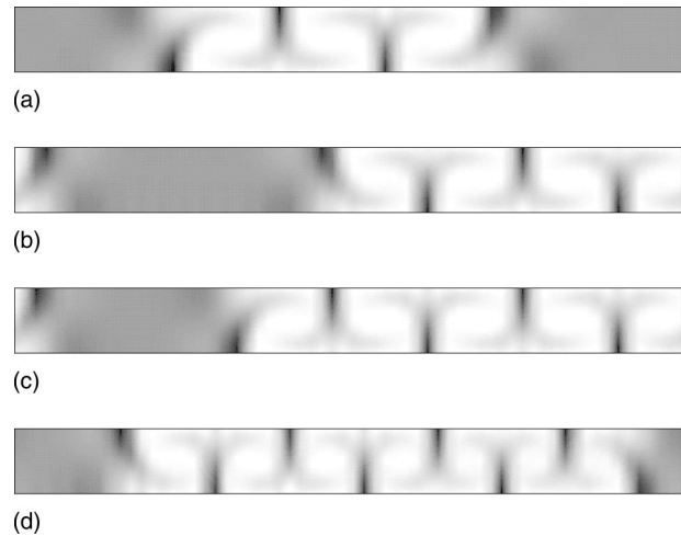
FIG. 1. Stable, stationary solutions for two-dimensional magnetoconvection, showing grayscale images of total magnetic field strength. Parameters are \sigma = 1, \zeta = 0.6, Q = 100 , and the Rayleigh and Nusselt numbers are (a) R = 2700, N = 1.75 , (b) R = 2800, N = 1.91 , (c) R = 3500, N = 2.19 , (d) R = 4000, N = 2.36 .
